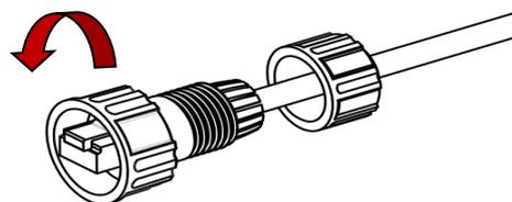
3. Tighten the sealing nut at the tail of the waterproof terminal.
