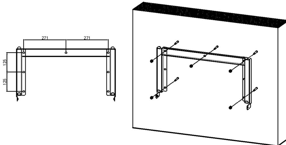
4. Attach the inverter to the wall mounting bracket. Screw the inverter to the wall mounting bracket on both sides using the M5 screws provided. Tighten the screws and make sure that they are securely in place.
