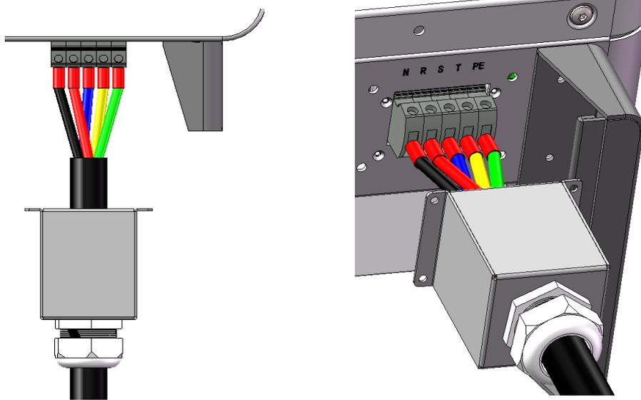
3. Combine the shell and the AC terminal of inverter with the combination screws M4 x 10.
