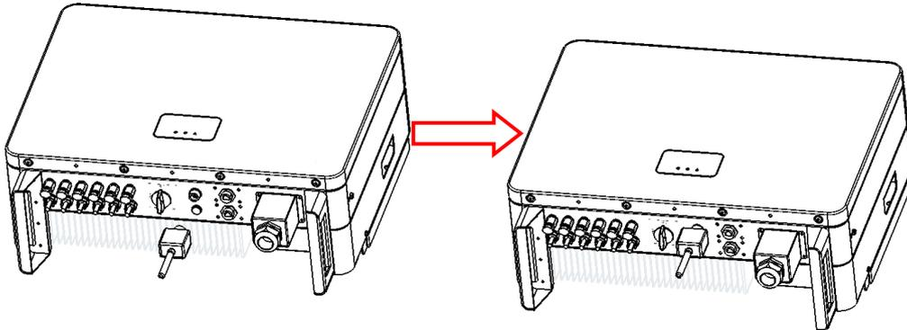
The RJ45 plug for electric meter communication and digital input is inserted into the COM2 connector, the RJ45 plug for DRM communication is inserted into the COM3 connector (only for Australian configuration).
