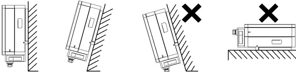
In order to maintain sufficient ventilation, when installing the inverter a minimum clearance of 30 cm at the sides and 50 cm at the top must be maintained. Operation and reading are made easier by installing the inverter with its display at eye level and by keeping a distance of 100 cm from the front. All cables are routed to the outside through the underside of the enclosure, therefore a minimum clearance of 50 cm must be observed here.
