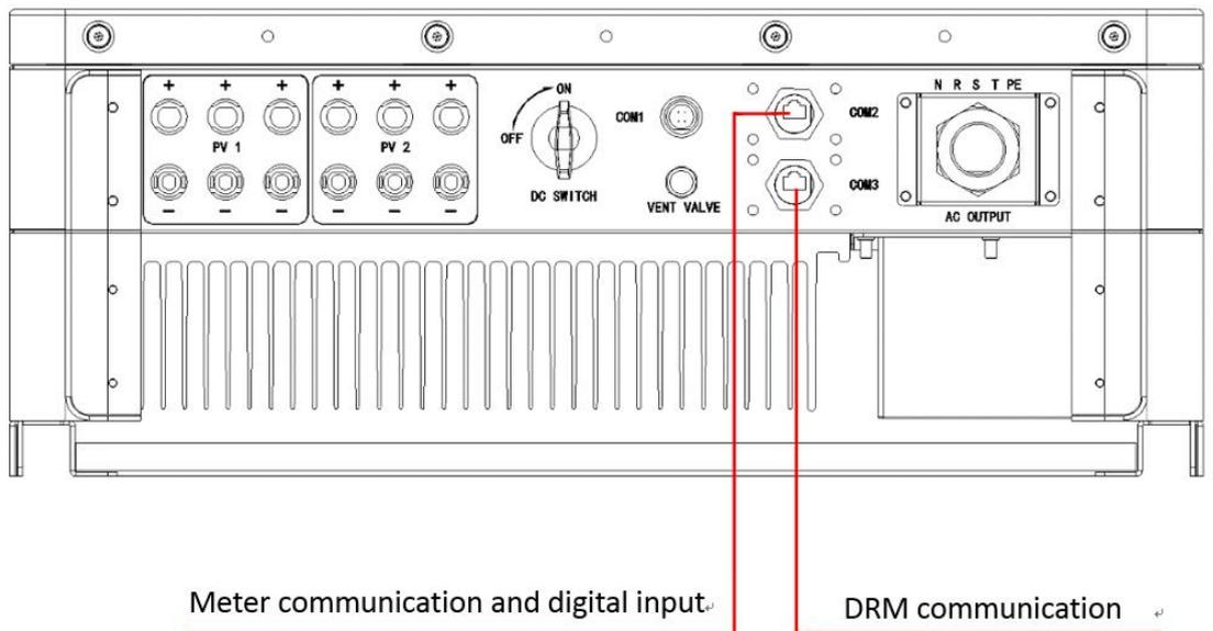
The enlarged image of the meter communication interface and DRM communication interface is as shown below:
