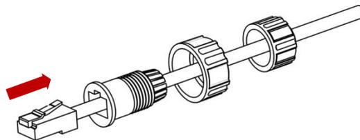
2. Insert the RJ45 crystal plug into the RJ45 port at the bottom of the inverter chassis then tighten the screw nut.
