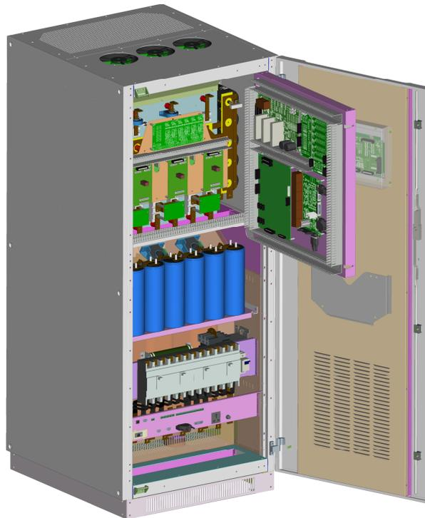
Figure 2-20: 80 ~ 120KVA UPS Physical Model of Internal Door
